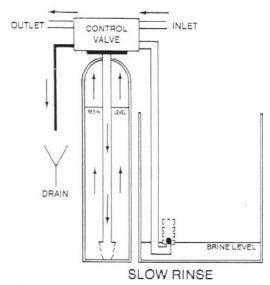
The slow rinse cycle position directs a slow flow of water down through the riser tube and up through the resin bed to drain. This slow flow of water pushes the brine solution through the resin bed
