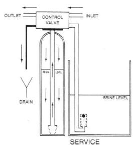
The service cycle position directs untreated water to flow down through the resin bed in the mineral tank and up through the riser tube. The water is conditioned when passing through the resin.
