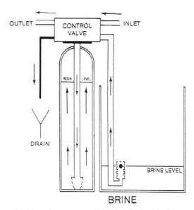
In brine draw, concentrated salt brine is drawn from the brine tank and directed to flow down through the riser tube and up through the resin bed to the drain. Brine is drawn until the air check in the brine tank closes.
